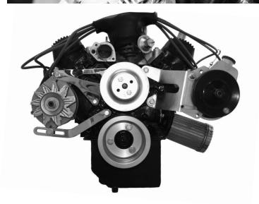
351W front view with correct water pump (note pass side water inlet) and brackets.
